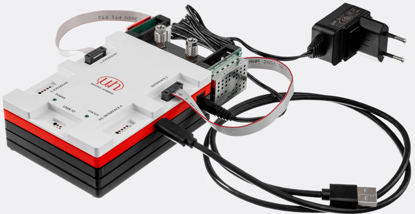
Micro-Hybrid Evaluation Kit "eNDIRi2" for IR components
